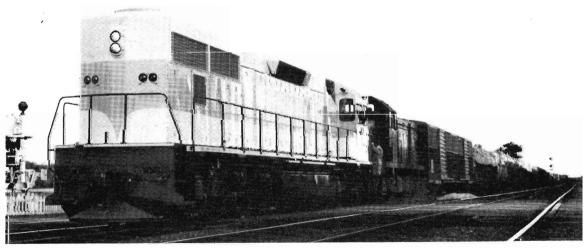
The W.A.G.R. 3,000/3,300 h.p. diesel on test run near Somerton
