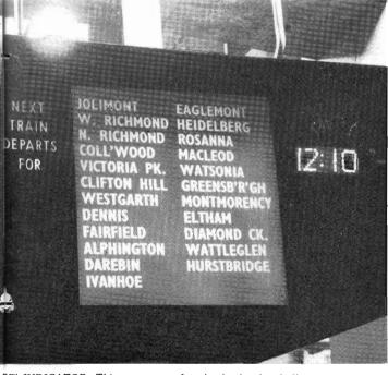
W INDICATOR: This new type of train destination indicator, recently fialled at Princes Bridge, uses rear projection of 35 mm. slides on to a ground ss screen. The departure times are shown on a digital clock that is illumated from a grid of neon lamps behind the glass screen. The indicator was ated from a grid of neon lamps behind the glass screen. The indicator was veloped by the Electrical Engineering Branch. (See News Letter, page 172, November 1965).
