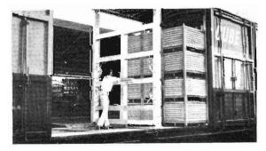
Load protection frame being placed in position in Hy-Cube van loaded with motor car parts.
