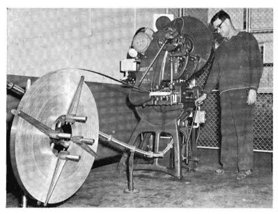
Using an automatic press, Machinist F. W. Broeder punches ticket blanks from aluminium strip.
