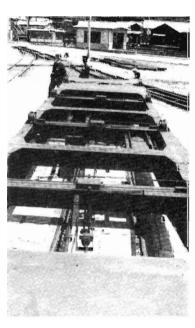
J.N.R. container wagon designed to carry five standard containers. As can be seen, this vehicle has no floor.
