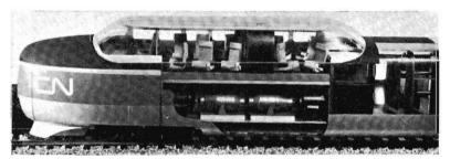
Model of a motor carriage of gas turbine train for the Canadian National Railways. Capable of speeds up to 160 m.p.h., the trains will give a fast and frequent service between Montreal and Toronto. The first two will be delivered in April, this year.
