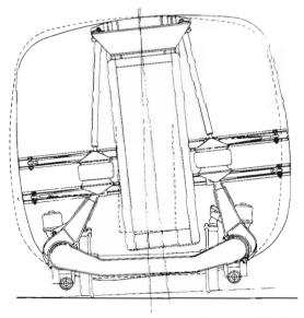
Diagram of suspension system for Canadian National Railways gas turbine trains. This suspension is designed to minimize swaying and lurching of train on curves. As seen from the end of the carriage, the unbroken line shows the outline of a carriage fitted with conventional suspension, as it would be positioned when taking a curve. With the pendulum type suspension, the body takes up the position shown by dotted line.
