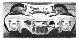
Aligned freight bogie. Note longitudinal side anchor and new type central bearing. Disc brakes as shown on this bogie were not common on freight vehicles.
