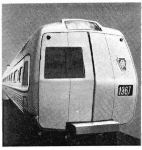
Mock up of a self-propelled, electrically driven, multipleunit rail-car ordered by the Pennsylvania Railroad Co. to attract passenger traffic for its New York-Washington service. Fifty will be required at a cost of over \$US400,000
