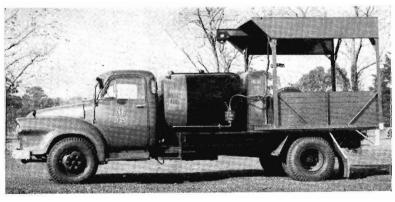
The V.R. motor truck that serves tractors with fuel, etc.
