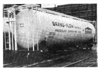
Among special wagons developed in U.S.A. to facilitate bulk handling is this Granu-Flow wagon that has inflatable, rubber-coated diaphragms inside. When inflated, the diaphragms break up compacted loads and channel the contents towards discharge outlets for fast unloading.
