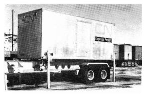
C.N.R. standard 20 ft. container on temporary legs so that road transport may be positioned under it. This type of container is usually loaded by a side loading unit.
