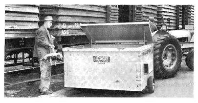
This type of container is designed to be hauled along a rake of wagons by tractor.
