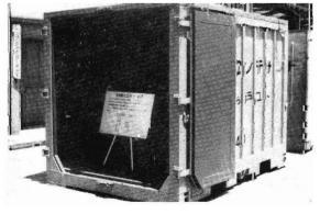
Special type of Japanese container. While of standard dimensions this 5-ton container is fitted with a removable roof.
