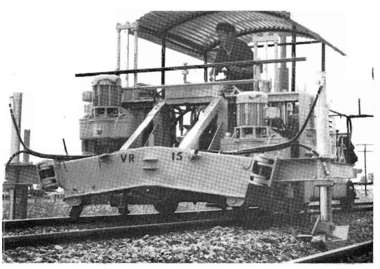
NEW TRACK MACHINE: One of the three medium class electromatic tamping machines that were recently delivered. They have in-built, manually controlled, hydraulic jacking and levelling devices, and an automatic tamping cycle. (See News Letter, page 10, January 1967).
