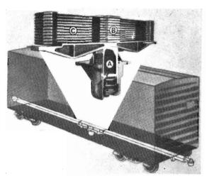
Diagram of hydraulic cushioning device of Hydra-Cushion
