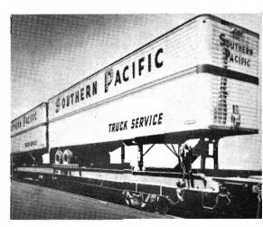
Piggy-back wagon showing retractable trailer hitch supporting front end of road semi-trailer.
