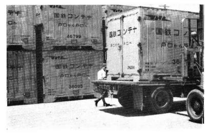
Standard containers at Umeda Yard, Osaka. These are 10 ft. 9 in. x 7 ft. 9 in. x 7 ft. 9 in. x 7 ft. 9 in. with doors at one end only. Note loading by fork lift truck. It will be seen from the dints that the containers must be robust to withstand normal usage.
