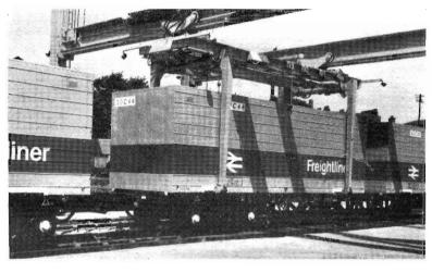
A 27-ft. container on British Railways. Note frame arranged to lift container from the bottom.
