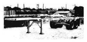
Light semi-trailer unit used for transport and storage of 40-ft. containers on Southern Pacific Railways.
