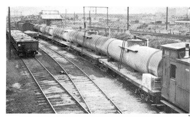
WATER TRAIN: Ready for instant dispatch when needed, the 50,000-gal, water train is shown standing at North Melbourne. Water from the train can be pumped into road vehicles at the rate of 22,000 gal, an hour. The two pumps also enable the tankers to refill from a river or stream close to the railway line instead of the train having to return to a railway location with watering facilities.
